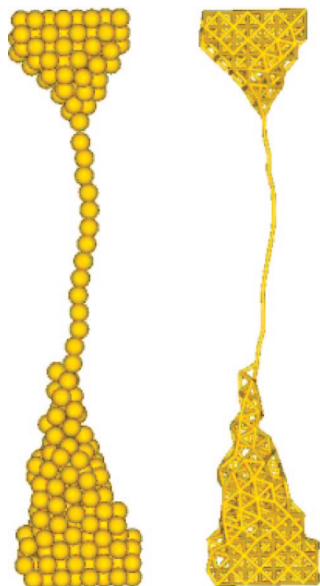
Figure 7. At 300 K, very long monatomic chain is formed for Au 256 when the elongation rate is increased to 5 m/s. The disordered structure at the two end contacts of the monatomic chain also indicates the high energy state of this structure.
